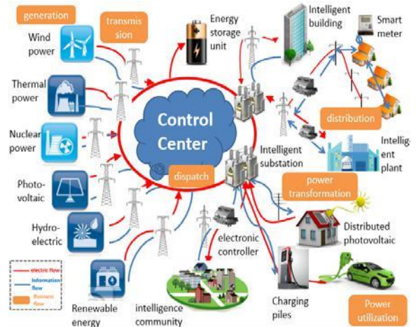
Figure 1 Tri-flows integration in Smart Grid
