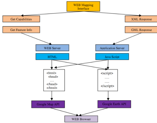
Figure 22. Diagram of develop the pseudo 3D map's application on Web browser
