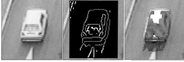
Figure 2.4: Left image: original, center: edges, right: optical flow [9].
