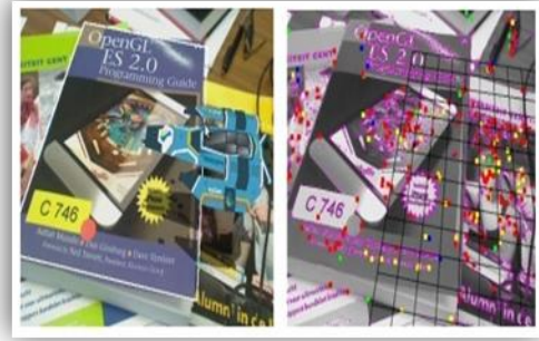
Figure 26. Augmented Reality application monitoring point specifies in video frames (right) to activate the coating 3D objects (left)
